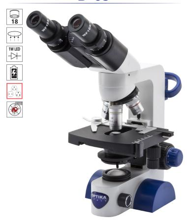
Cordless, modern binocular microscope ideal for students and mainly primary schools with achromatic lenses (1000x), FN 18 eyepieces, finite optical system, coaxial focusing, StagErase™ eraseable mechanical stage, Abbe condenser and 1 W LED illumination with rechargeable batteries. Slim and easy to carry, it is equipped with arm/wrist rest support to reduce the fatigue during use and long lasting LED illumination to provide over 20 years of use
